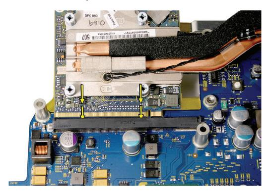
2. Install the three screws and connect the sensor cable to the logic board. **Replacement Note**: The shorter screw attaches at the far right end of the video card heatsink.
